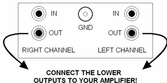
Make sure the connectors are pushed all the way in. If they are too loose or too tight, the music will suffer. If possible, try tightening or loosening the male connectors of your interconnect until the fit is “just right”. If your turntable has a ground lead,
