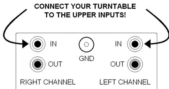
Now connect a good pair of interconnects from the outputs to a pair of line level inputs on your amplifier as shown below.
